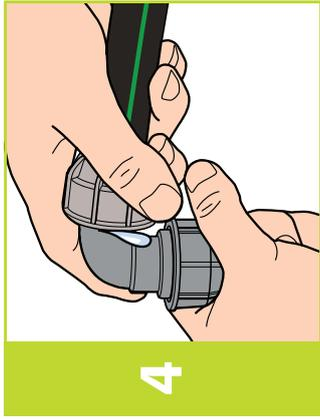
Ensure the pipe connections are tight, otherwise pump will not pressurise.
