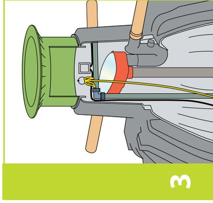
Lower pump into tank using the nylon cord **(C)**, ensure pump is seated firmly on the floor of the tank.
