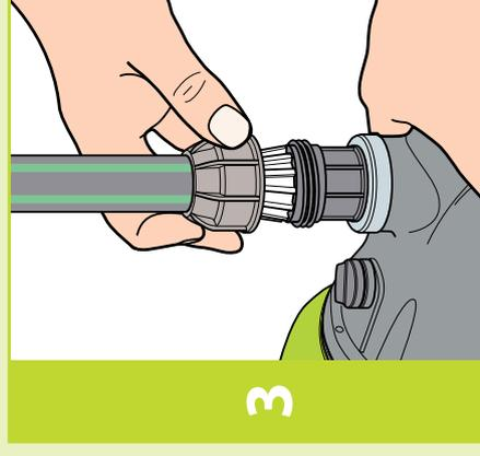
Connect output pipe into the outlet connector **(B)**.
