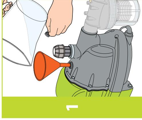
Fit a cartridge filter to the input of the pump. Remove filler screw **(A)**, fill with water (about 2 litres) and replace tightly.
