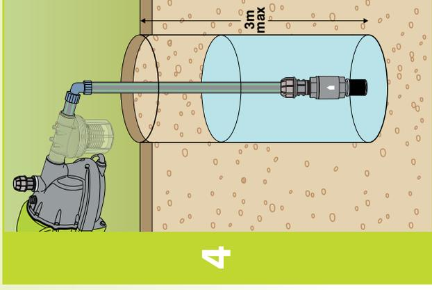
If the pump is drawing water from a lower level, fit a non return valve (not supplied) on the inlet pipe at its lowest point. Prior to first pumping, fill the pipe with water.
