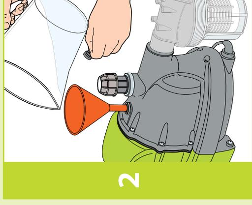
Remove filler screw **(A)**, fill with water (about 2 litres) and replace tightly.
