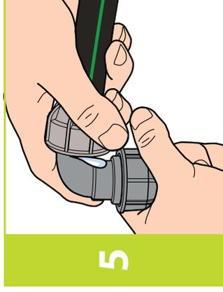
Ensure the pipe connections are tight.
