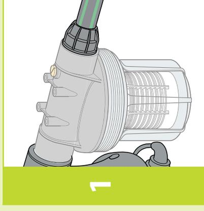
Connect your input pipe and optional cartridge filter (neither supplied) to the pump inlet which has a 1" BSP male thread.
