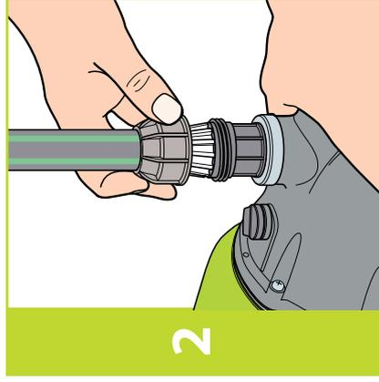
Connect output pipe into the outlet connector **(B)**.
